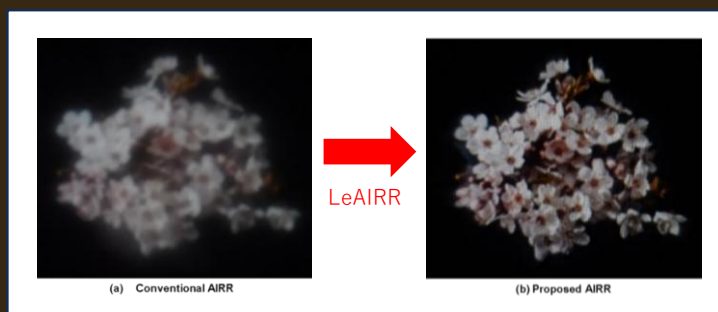
Fig. 3 High-resolution aerial imaging using lens-enhanced aerial imaging by retro-reflection (LeAIRR).
