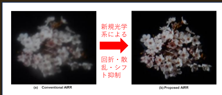
図3. レンズ増強AIRR(LeAIRR: lens-enhanced aerial imaging by retro-reflection)による高解像度化
